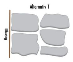
Minimal adjustment creates gaps of 5-15 cm, which can be filled with gravel, sand, stone chips, river stones, soil, or grass seed.
