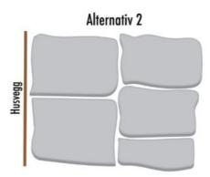
A higher degree of customization for a cleaner look results in joints between 2–5 cm, which can be filled with materials like subbase/sand, soil, and grass seeds.
